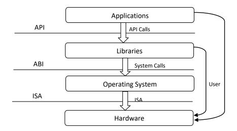
Figure 2.4 Machine reference model
