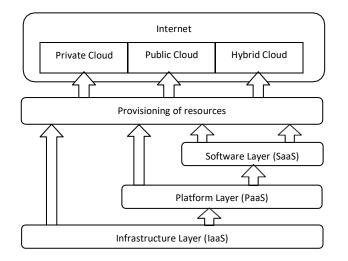
1. Illustrate architecture of a cloud is developed using three layers.
