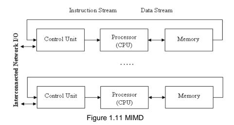
MIMD systems are broadly categorized into shared memory MIMD and distributed memory MIMD based on the way processing elements are coupled to the main memory.
