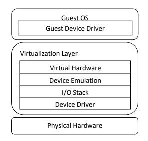
Figure 2.10 Device emulation for I/O Virtualization
